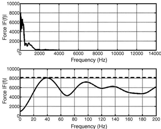
**Fig 6.** Fourier-transformed NMI force-time history (maximum setting, test 005). The upper graph shows the force amplitude over a frequency range 0.38 Hz to 12.5 kHz. The lower graph shows the frequency response up to 200 Hz for which the dynamic force amplitude area ratio and energy were 69.5% and 1120 kN Hz, respectively. See text for definitions of dynamic area ratio and energy.
