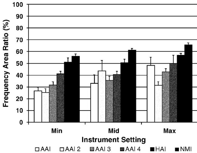
**Fig 9.** Mean frequency area ratio comparison of the five chiropractic adjusting devices, the AAI, AAI 2, AAI 3, AAI 4, and the electromechanical devices, the HAI and the NMI, at the respective maximum, middle, and minimum force settings. Settings 2, 3, and 4 are presented for the AAI 4. Error bars represent standard deviations of the mean.
