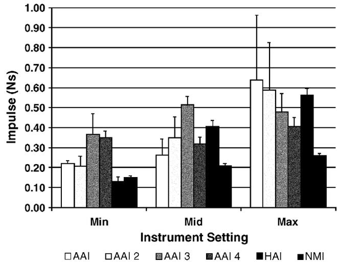
**Fig 11.** Mean impulse comparison of the five chiropractic adjusting devices, the AAI, AAI 2, AAI 3, AAI 4, and the electromechanical devices, the HAI and the NMI, at the respective maximum, middle, and minimum force settings. Settings 2, 3, and 4 are presented for the AAI 4. Error bars represent standard deviations of the mean.
