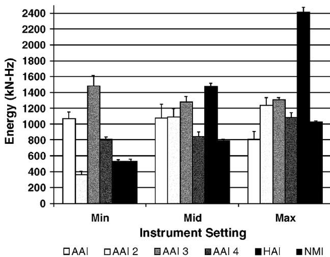
**Fig 10.** Mean energy comparison of the five chiropractic adjusting devices, the AAI, AAI 2, AAI 3, AAI 4, and the electromechanical devices, the HAI and the NMI, at the respective maximum, middle, and minimum force settings. Settings 2, 3, and 4 are presented for the AAI 4. Error bars represent standard deviations of the mean.
