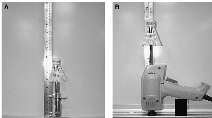
**Fig 2.** The AAI 2 (A) and HAI (B) were attached rigidly and vertically to a frame with a ruler in the background. A shuttlecock was ejected by these instruments, and the height of flight in centimeters and the duration of flight in seconds were measured by video.
