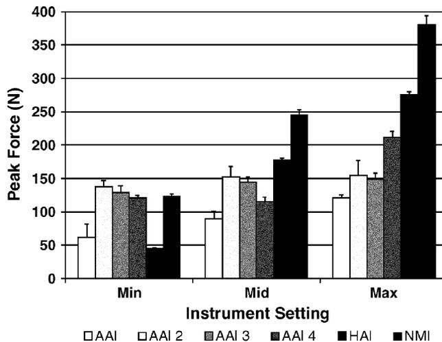
**Fig 8.** Mean peak force comparison of the six chiropractic adjusting devices, the AAI, AAI 2, AAI 3, AAI 4, and the electromechanical devices, the HAI and the NMI, at the respective maximum (max), middle (mid), and minimum (min) force settings. Settings 2, 3, and 4 are presented for the AAI 4. Error bars represent standard deviations of the mean.
