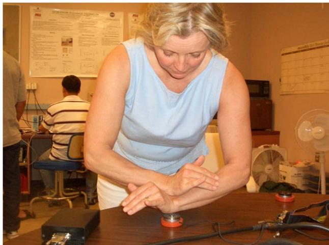
**Fig 1.** A clinician applies a McTimoney technique thrust into a table-top mounted load cell.
