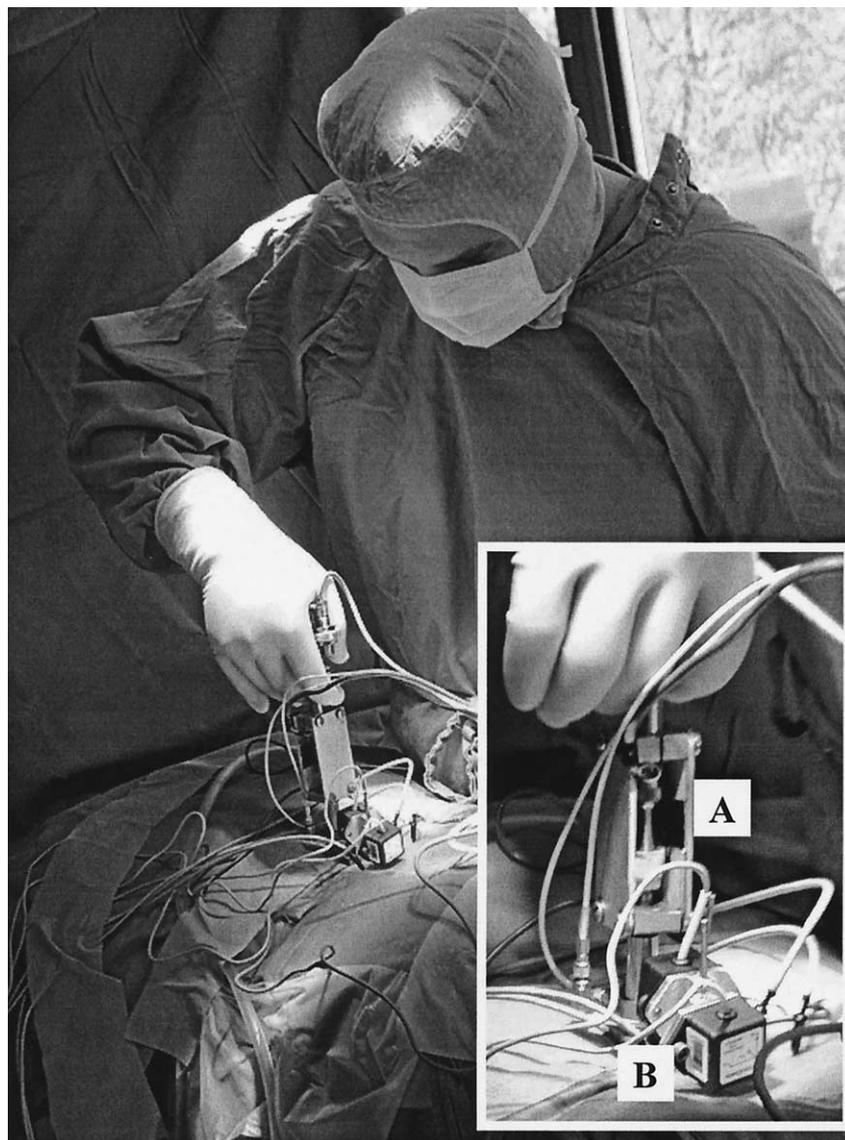
**Fig 1.** Experimental protocol noting surgical preparation (patient 003) with detail of the AAI instrumented with preload control frame, force and acceleration transducers (A), and the 3-axis accelerometers affixed to the intraosseous pins (B).
